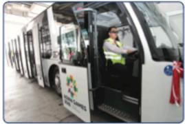
An apron bus with a capacity of 105 people serves the process of moving passengers from the aircraft to the terminal or vice versa.
